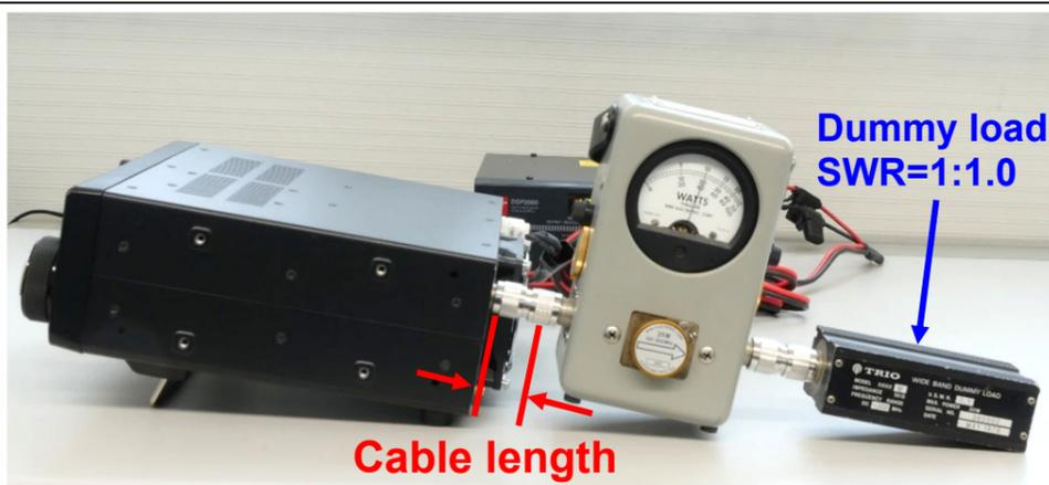
RF power is set at 10 W with a 50  $\Omega$  dummy load.
